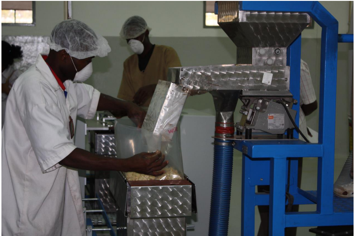
Figure 9.9: Vacuum packaging of kernels Source: GIZ/ComCashew
