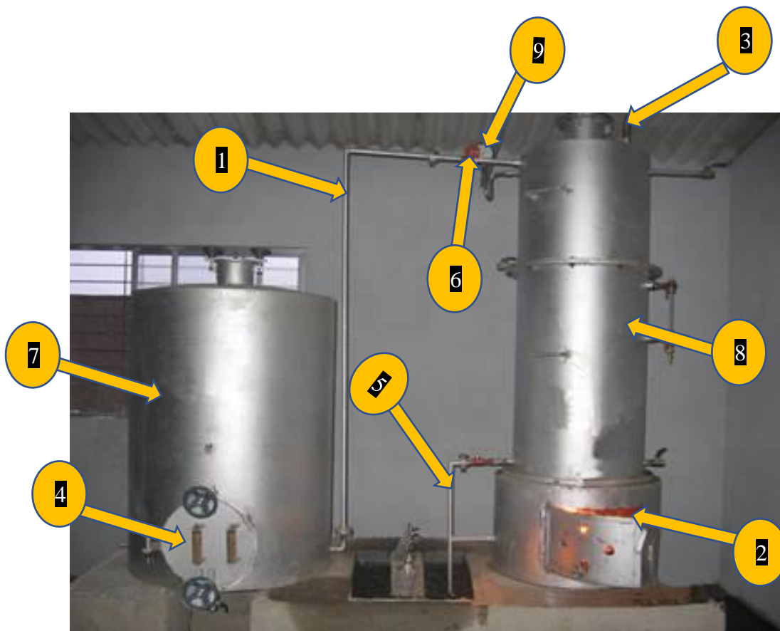
Figure 8.3. Steam Cooker and Boiler
