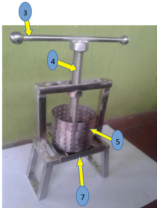
Figure 7.1. Mechanised Juice extractor – Screw Press. Source: http://www.intermech.ws/products.htm
