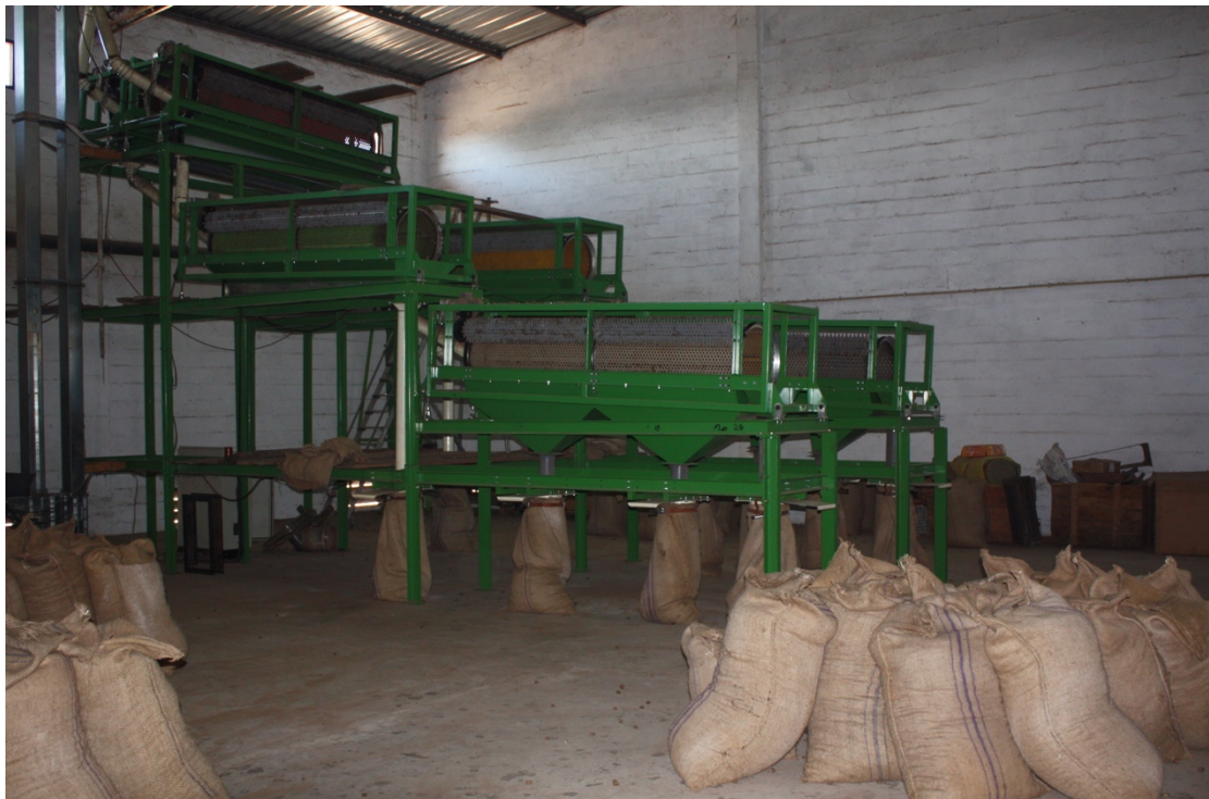
Source: GIZ/ComCashew – Calibrating raw cashew nuts and bagging in jute bags
