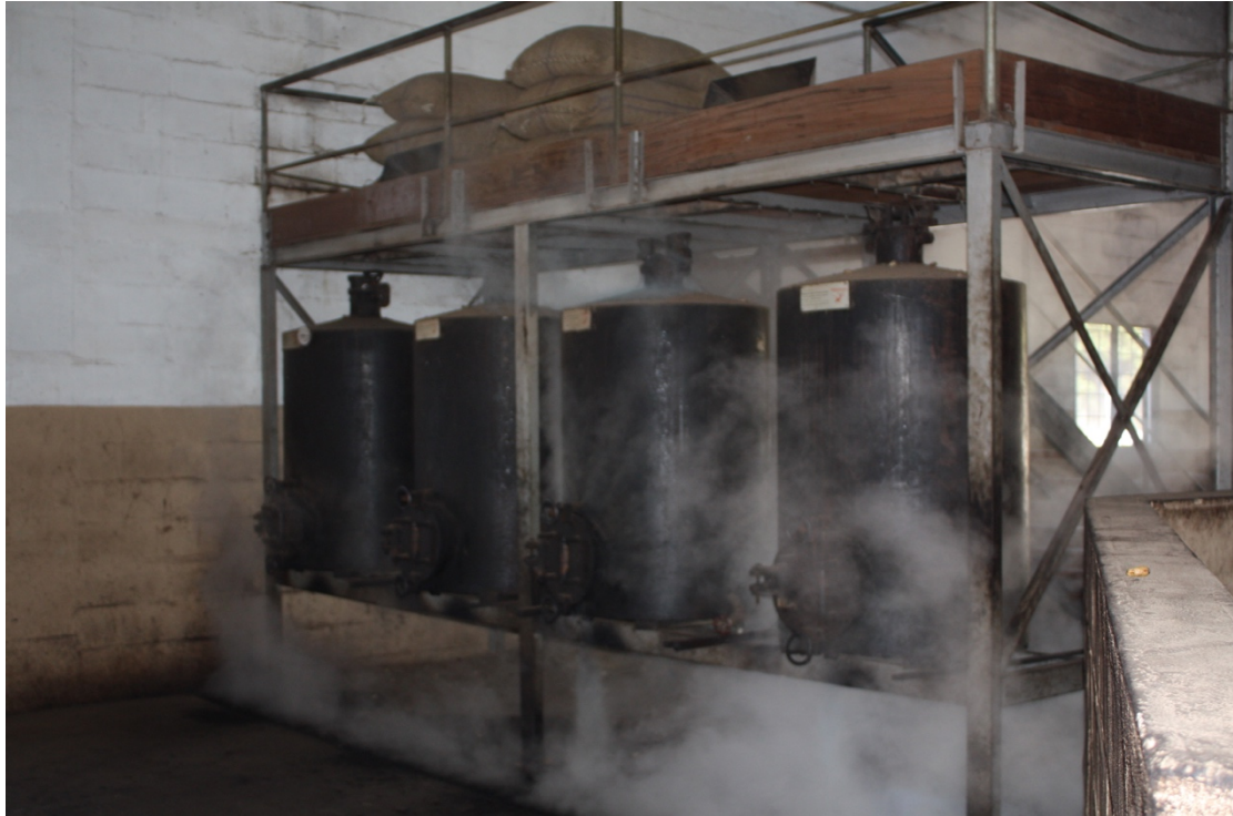
Source: GIZ/ComCashew – Steaming of raw cashew nuts in preparation for de-shelling
