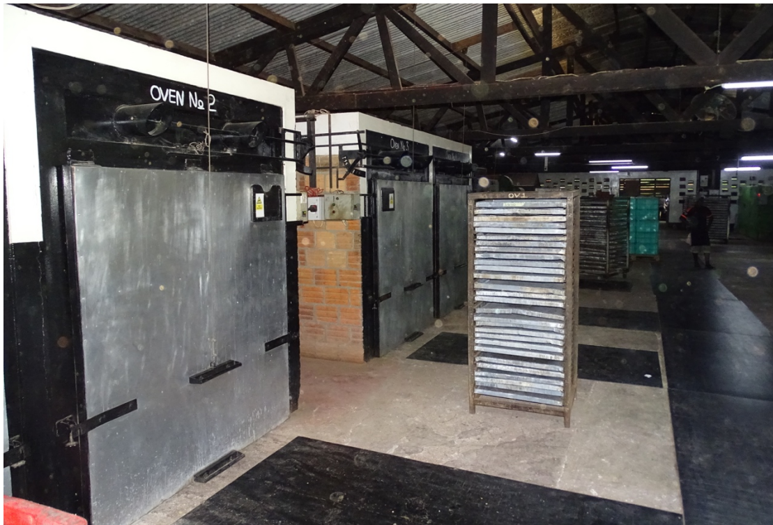
Source: GIZ/ComCashew – Oven drying in cashew processing factory
