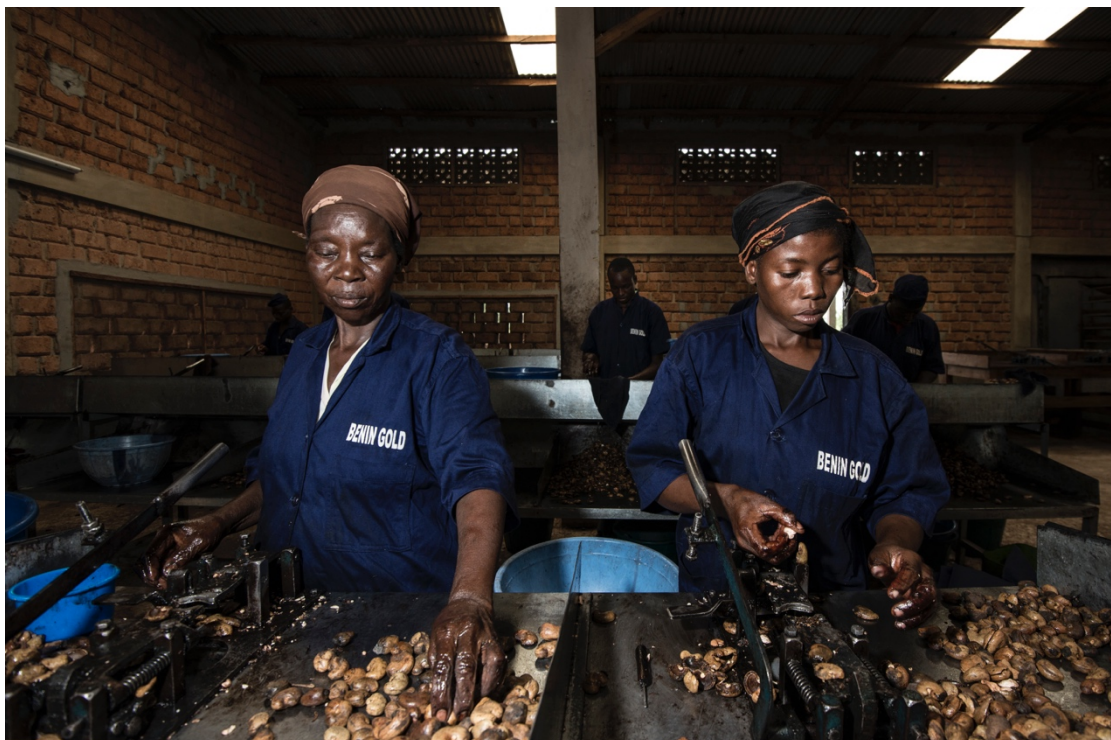
Source: GIZ/ComCashew – Manual de-shelling in cashew processing factory
