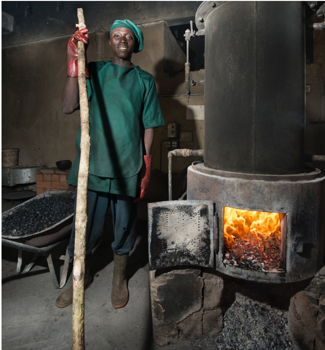
Source: GIZ/ComCashew – Firing steamer for heat treatment of raw cashew nuts
