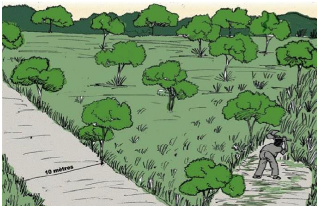
Source: GIZ/ComCashew – Fire belt construction around a plantation
